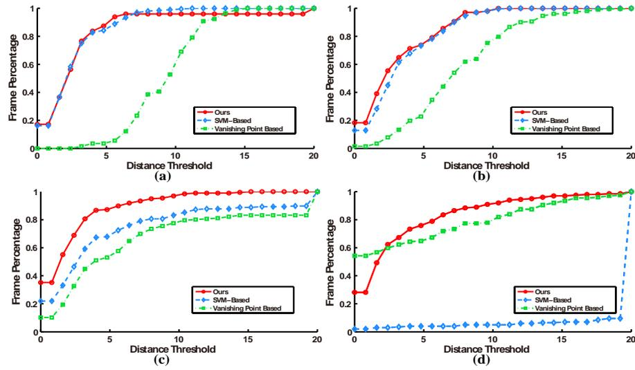
Figure 10: Evaluation of the proposed method with two competitors by *vanishing point distance*. After road detection, each detected vanishing point has a distance from the ground truth one. Then we set different thresholds (horizontal axis) to count the percentage of frames (vertical axis) with a smaller distance than the threshold. (a)-(d) are respectively the results of the four road scenes.
