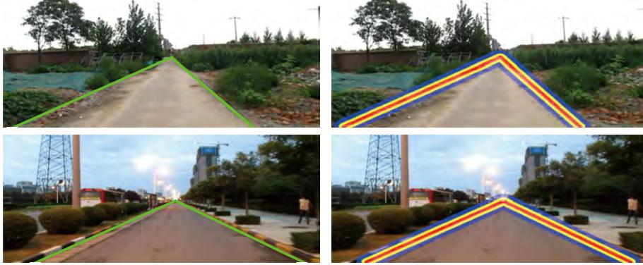
Figure 3: Illustration of training sample selection. For the left images, the green lines indicate the ground truth road boundary. For the right images, positive instances can be randomly selected from the red region and negative ones from the blue region. The yellow region is served as a transition area.
