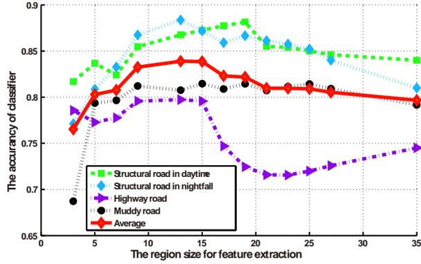
Figure 5: The performance under different patch size for feature extraction of the sample instance. The horizontal axis is the patch size  $N$ , and the vertical axis is the accuracy of the classifier.
