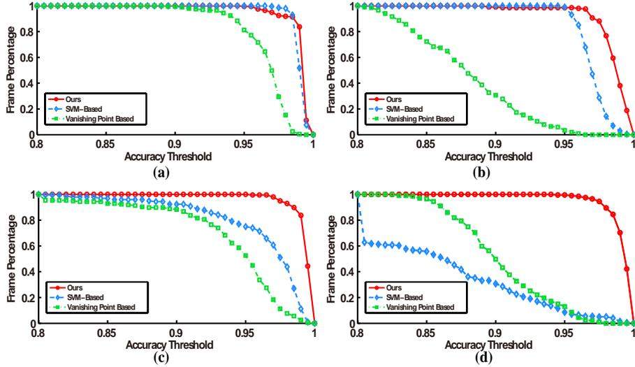
Figure 9: Evaluation of the proposed method with two competitors by *road region accuracy*. After road detection, each frame has an accuracy according to the ground truth labelings. Then we set different thresholds (horizontal axis) to count the percentage of frames (vertical axis) with a higher accuracy above the threshold. (a)-(d) are respectively the results of the four road scenes.
