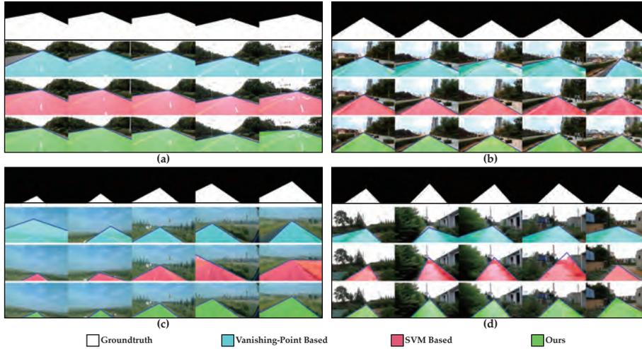
Figure 8: Typical road detection results of the vanishing-point based, SVM based, and the proposed method in this paper. The four kinds of scenes are separately showed in (a), (b), (c), and(d). For each scene, from top to bottom are the ground truth, the results of two competitors and our method.
